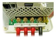
**Up to 3 isolated outputs.** Each output can carry the full current rating of the charger. However, not all simultaneously - the total current is the charger's rating.
